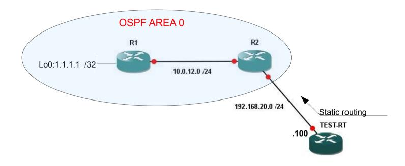
Each router has the point-to-point connection in format: 10.0.xy.z /24 where:
