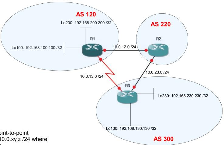
Each router has the point-to-point connection in format: 10.0.xy.z /24 where:
